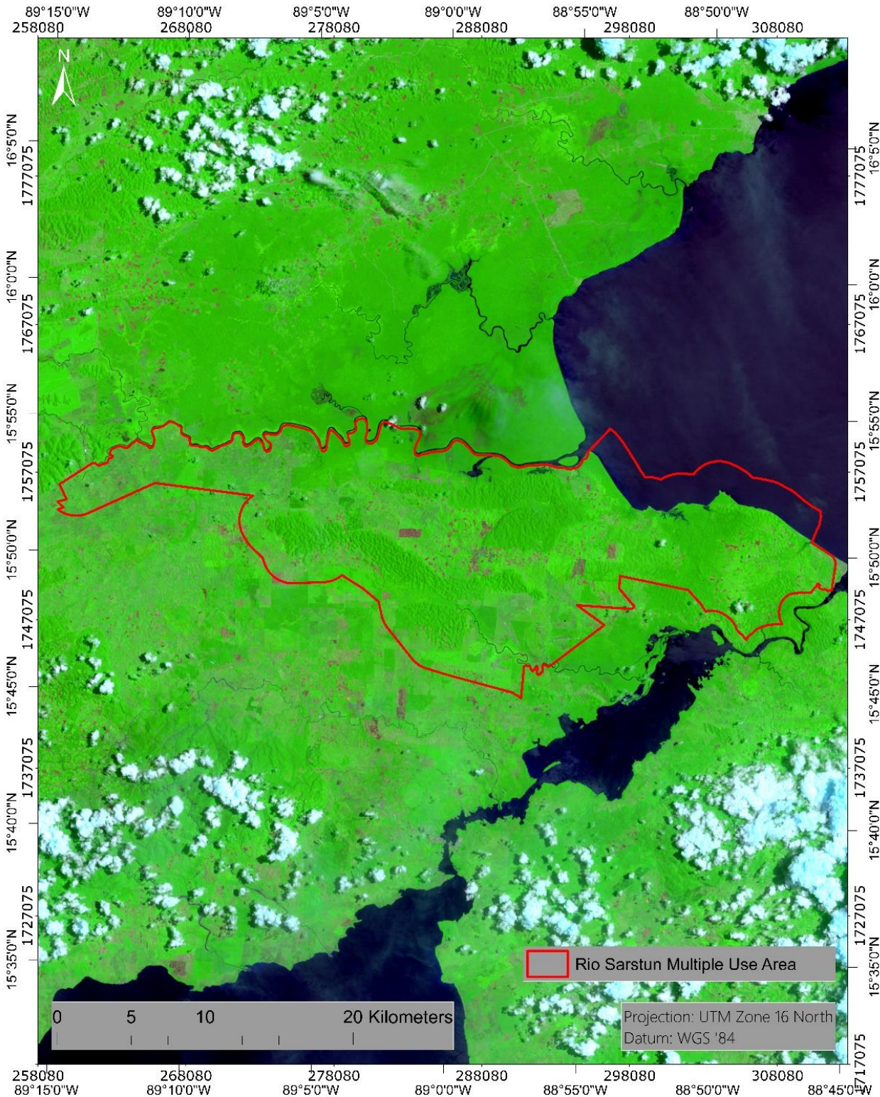
Figure 5: Landsat 8 scene (2018-05-17; bands: short wavelength infrared (band 7), near infrared (band 5), and red (band 4) used for the mangrove and seagrass mapping.
