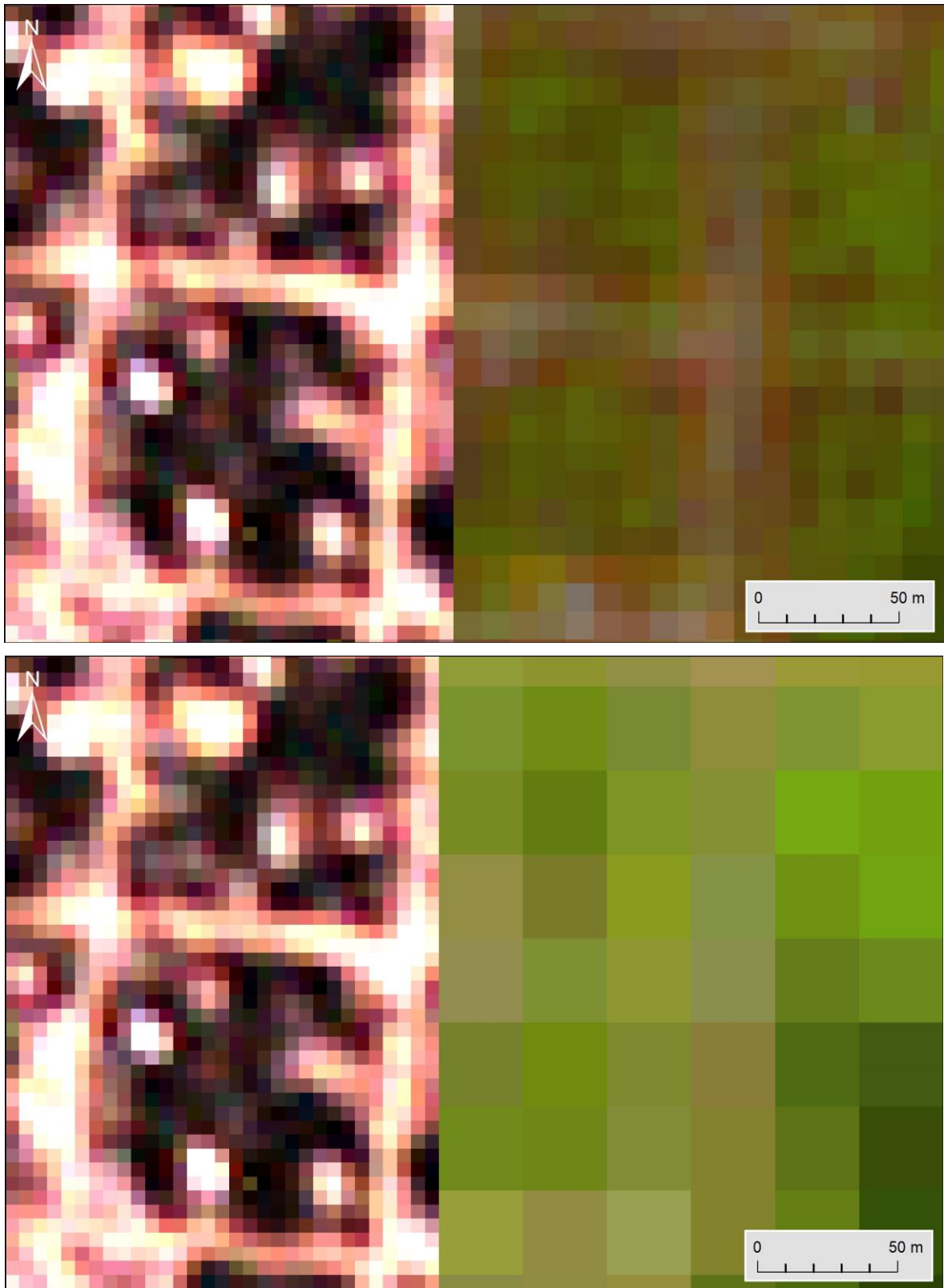
Figure 8: Geometrical fit of the Sentinel-2A data (upper figure right) and Landsat 8 data (lower figure right) in comparison to RapidEye data (upper figure left and lower figure left). Exemplarily streets (permanent features) is shown. The streets are spatially located at the same location within all shown datasets. Additionally, the two figures show, that the pixels exactly fit to each other. Due to this no geometrical co-registration was necessary.
