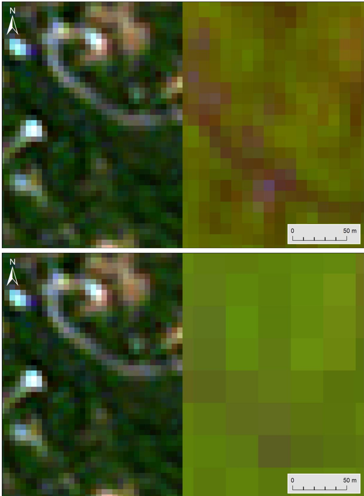
Figure 8: Geometrical fit of the Sentinel-2A data (upper figure right) and Landsat 8 data (lower figure right) in comparison to RapidEye data (upper figure left and lower figure left). Exemplarily a street (permanent feature) is shown. The street is spatially located at the same location within all shown datasets. Additionally, the two figures show, that the pixels exactly fit to each other. Due to this no geometrical co-registration was necessary.
