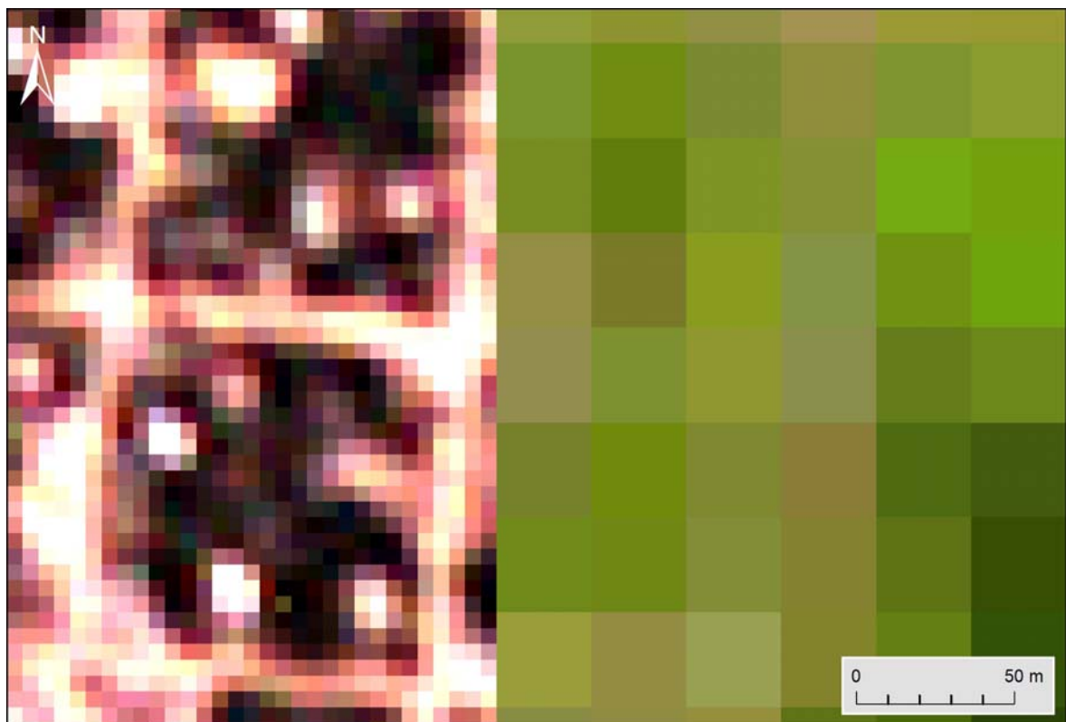
Figure 8: Geometrical fit of the Sentinel-2A data (upper figure right) and Landsat 8 data (lower figure right) in comparison to RapidEye data (upper figure left and lower figure left). Exemplarily streets (permanent features) is shown. The streets are spatially located at the same location within all shown datasets. Additionally, the two figures show, that the pixels exactly fit to each other. Due to this no geometrical co-registration was necessary.
