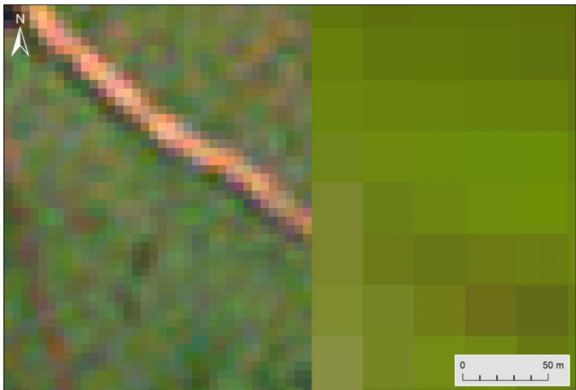
Figure 8: Geometrical fit of the Sentinel-2A data (upper figure right) and Landsat 8 data (lower figure right) in comparison to RapidEye data (upper figure left and lower figure left). Exemplarily a street (permanent feature) is shown. The street is spatially located at the same location within all shown datasets. Additionally, the two figures show, that the pixels exactly fit to each other. Due to this no geometrical co-registration was necessary.
